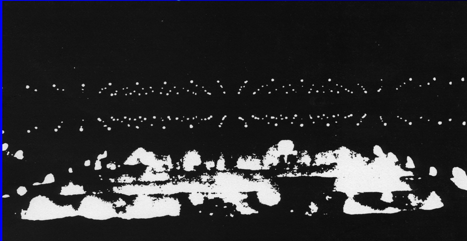
Back Corona Glow Regions on Collecting Plate Ash Surfaces Plan View – Looking Down Into a Gas Passage
